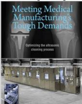
Many recent developments position ultrasonics as an ideal and sometimes the only answer to many of the challenges found in cleaning for the medical industry. This 13-stage system effectively handles medical implant cleaning and passivation.
