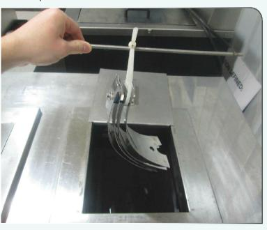
smaller diameter hole in the center at the top of the cone. These discs are constructed of thin stainless steel and have radial features that space the discs apart when nested in the centrifuge. These features also contribute to the separation efficiency of the centrifuge by interrupting and redirecting the flow of the material being processed.
