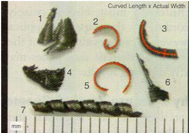
Figure 3. Software can be used to measure the curvilinear length of a particle, which accounts for the longest possible configuration in the event of flexing.
