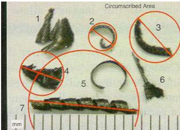
Figure 4. The circumscribed area is calculated by taking the long axis of a particle and forming a sphere, the area of which accounts for its circle of influence.
