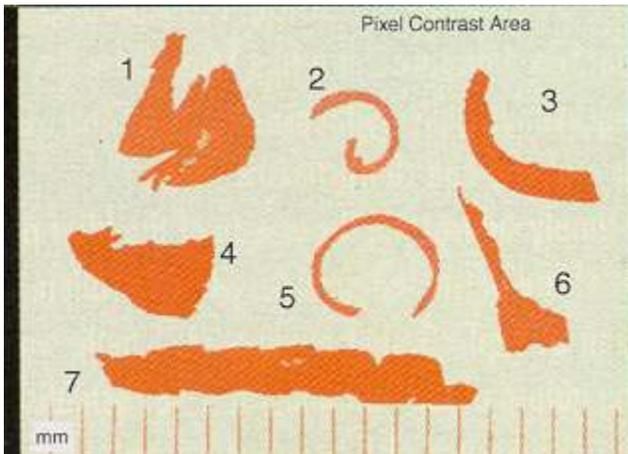
Figure 5. Computer software can use shade contrast and pixel count to quickly and accurately measure the size of a particle.
