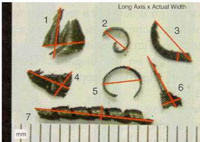
**Figure 2.** The long axis and cross section method of calculating the size of a particle is most useful for "C"-shaped chips and loops (Particles 2, 3, and 5).
