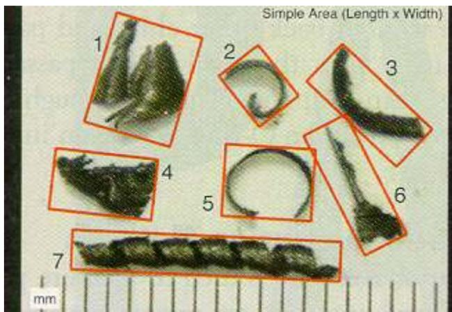
**Figure 1.** The simple area of a particle is determined by calculating the area of an imaginary rectangle around the particle.
